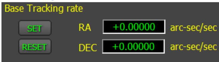
The base tracking rate is a constant tracking correction rate that is fixed during the observing run. If the mount has a known 'bias' in its tracking error then the base tracking rate correction can be used to offset that. Normally this value is set to 0.
