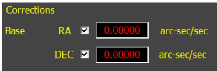
This is the base correction rate applied to the RA and DEC motors. It is a fixed value that is only changed by the user. To set or reset the base rate use the [Base Tracking Rate](#) on the config tab.
