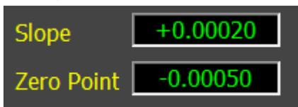
This is the slope and intercept of a straight line representing the tracking rate for a given hour angle along a declination arc. There is one set for the RA motor and another set for the DEC motor in each sky (East or West). These values are normally calculated by plotting the tracking correction rates from an ATrack log over a declination arc and then fitting a straight line to it. The intercept is the tracking rate at the meridian and the slope is the change in tracking rate by hour angle.
