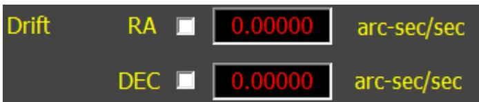
The drift rate is calculated by subtracting the plate solution from the previously solved image and the current solved image (see [Theory of Operation](#) for more detail).
