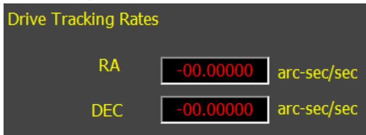
These are the current tracking rates received from the mount. It should include the sum of all the ATrack correction rates:
